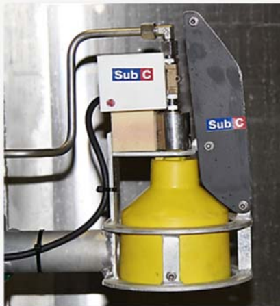
The gas sampler
